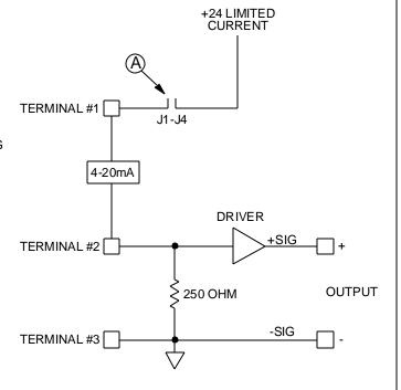
2 WIRE "SINKING" DEVICE CONNECTS TO TERMINALS 1 & 2
